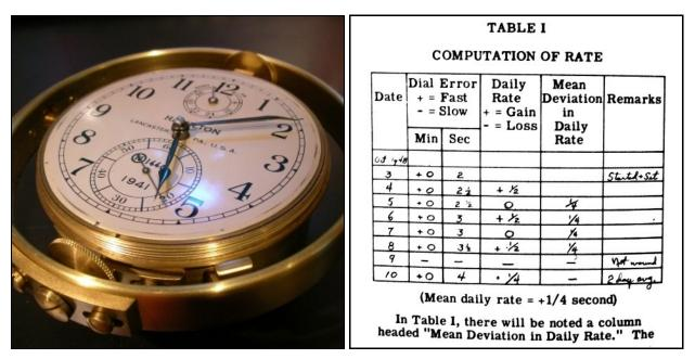
The photo on the left is a marine chronometer. On the right is a typical rate calibration chart:
