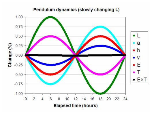
We see that in both cases, the black line,  $E \times T$ , is flat. So pendulum simulation scores another victory – it has confirmed that E times T is an adiabatic invariant, just like theory says. This is very satisfying. It's almost as if the entire universe is just a big fast simulator.
