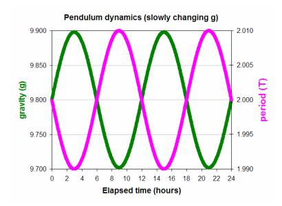
The plot shows that g varies from 9.7 to 9.9 m/s<sup>2</sup>, which is  $\pm 1\%$  of 9.8, as we specified. The simulation shows that T varies from 1.99 to 2.01 s, which is  $\pm 1/2\%$  of 2.0, and opposite phase as g.
