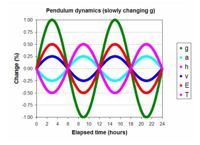
Note that amplitude changes in the opposite direction as velocity. That is, as gravity increases, velocity increases but amplitude decreases.
