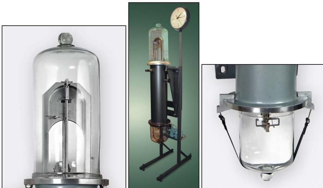
Like other clocks in its class, the features of the AChF-3 are that it runs in vacuum (5 mm Hg), has a 1 meter, 10 mm invar rod, small amplitude (100 arc-minutes), and a 10 kg temperature compensated copper bob with thermally exposed core. Two unique features are the isochronous triple spring suspension and electro-magnetic, transistor amplified sense/impulse coils, which are active once every period. This is all covered in great detail in Feinstein's paper.
