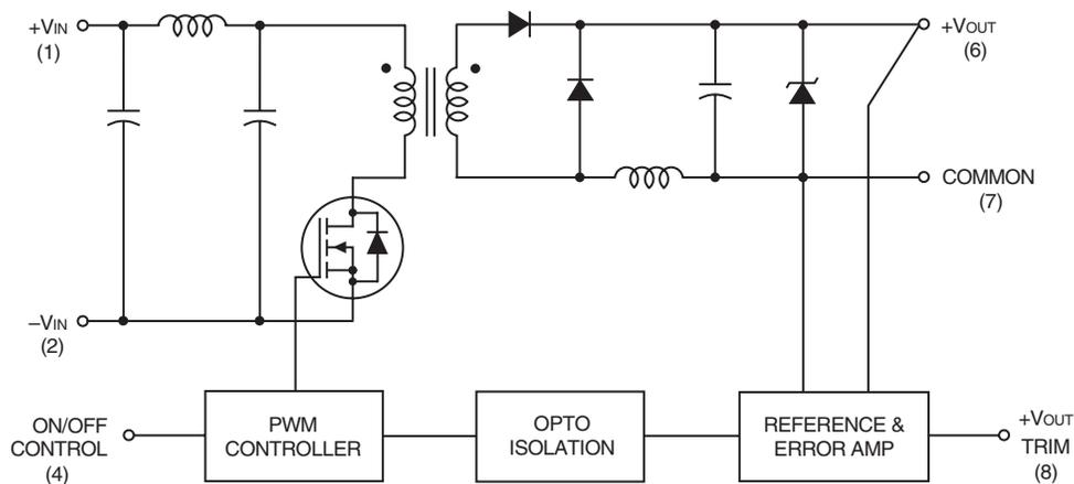
Figure 1. Simplified Schematic
