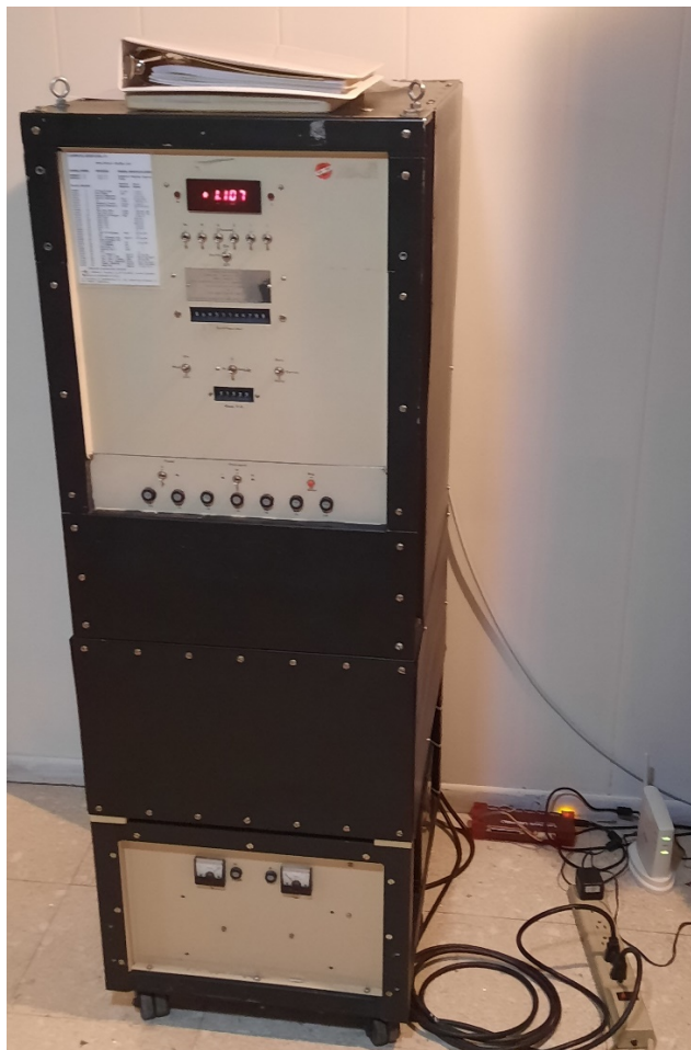
Photo 11 & Chart 1 – MHM-A1 is running again. Still a few screws to put in the covers. Have it running about 4ns slow over three days a little more than a week after first cavity register LOCK.
