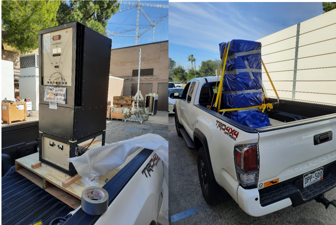
Photo 1 & 2 – MHM-A1 at JPL. You can see the wires hanging out the front, there was also a pot hanging out the back corner. It was palletized, wrapped in heavy plastic, packing blankets, and finally the blue tarp.
